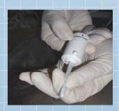
Secure "slider" to assure all air is removed
