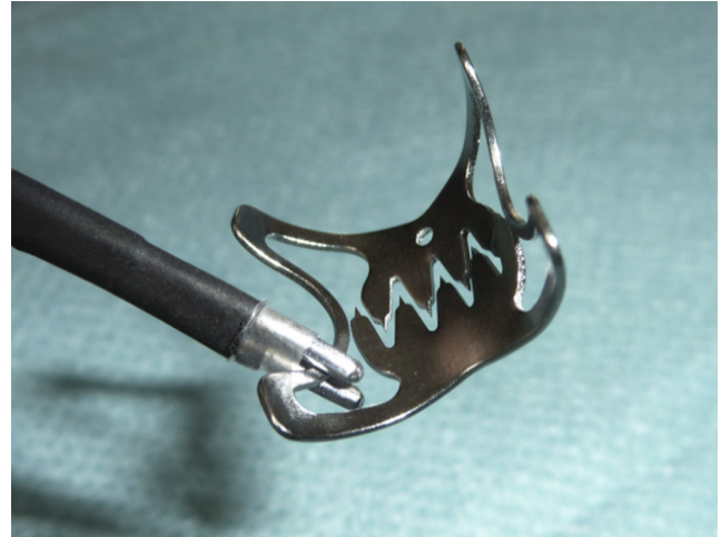
Supplementary Figure 2. The DC Clip Cutter (OVESCO). The DC ClipCutter is a monopolar grasping device that can be advanced through a 3.2-mm working channel. The nitinol of the over-the-scope clip (OTSC) is cut by application of a short direct current impulse.
